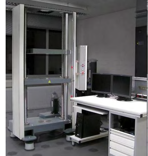
Materials testing Machine ZWICK Z050 – Characterization of the viscoelastic properties of substrates (foil, paper), blankets, flexographic printing plates, ...
